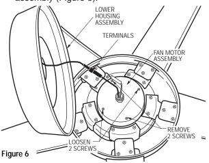
11. Attach the lower housing assembly to the fan motor using the two key slot holes. (Figure 7). Secure the lower housing assembly by tightening the two screws. Reinstall the two screws that were removed.
